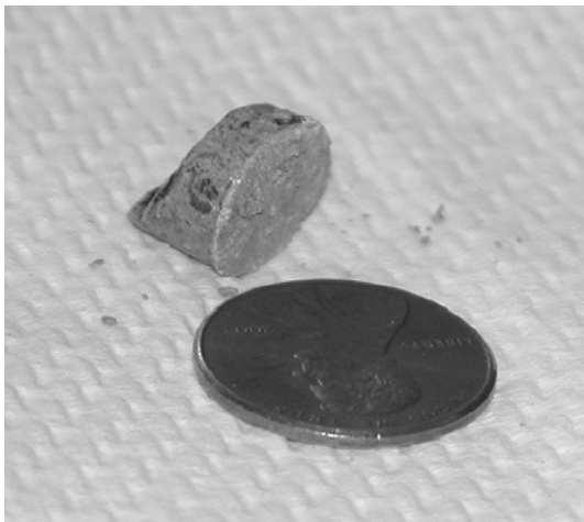
Fig. 2. Burial glass fragment exhumed after 24 years (a copper penny for scale).
